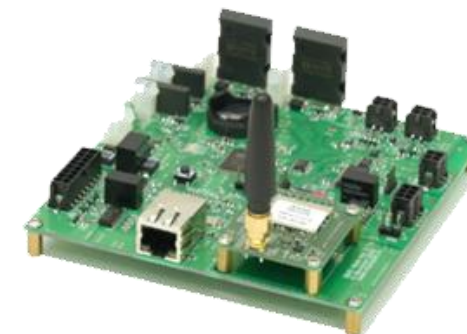
Battery Management System
